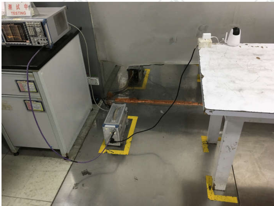
Conducted Emissions Test Setup
