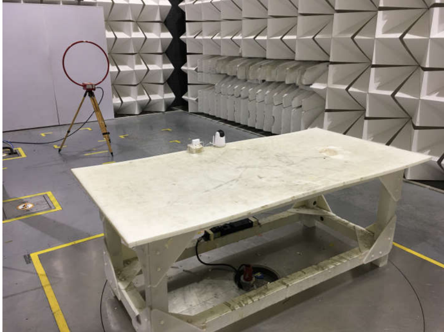
Radiated spurious emission Test Setup-1(Below 30MHz)
