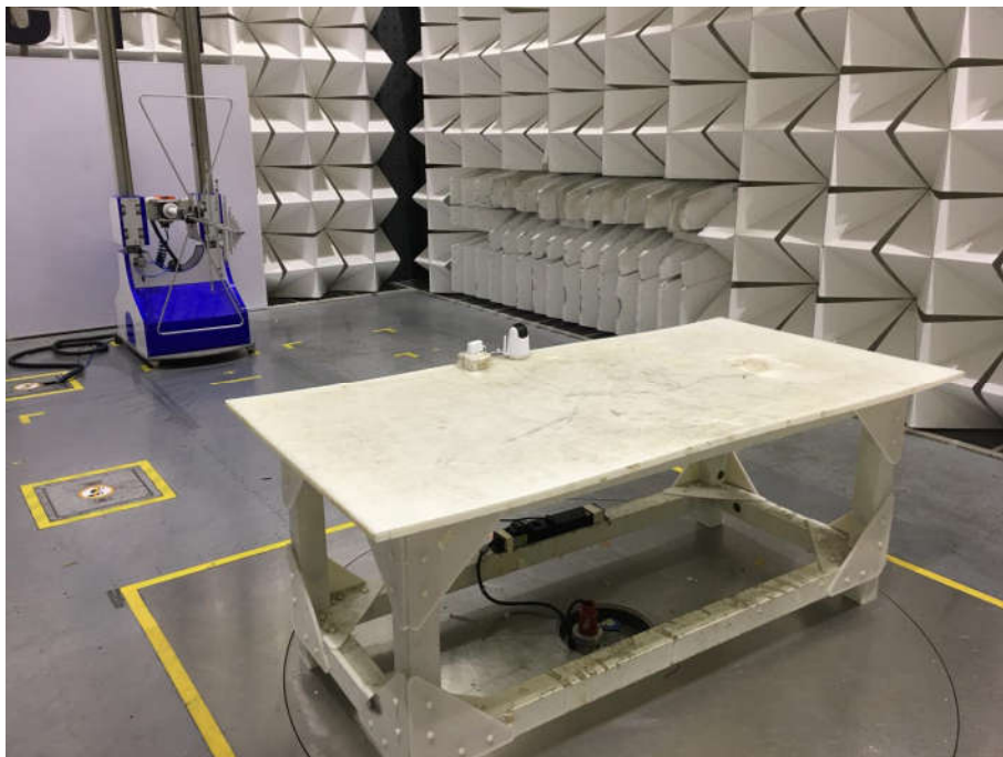
Radiated spurious emission Test Setup-2(Below 1GHz)
