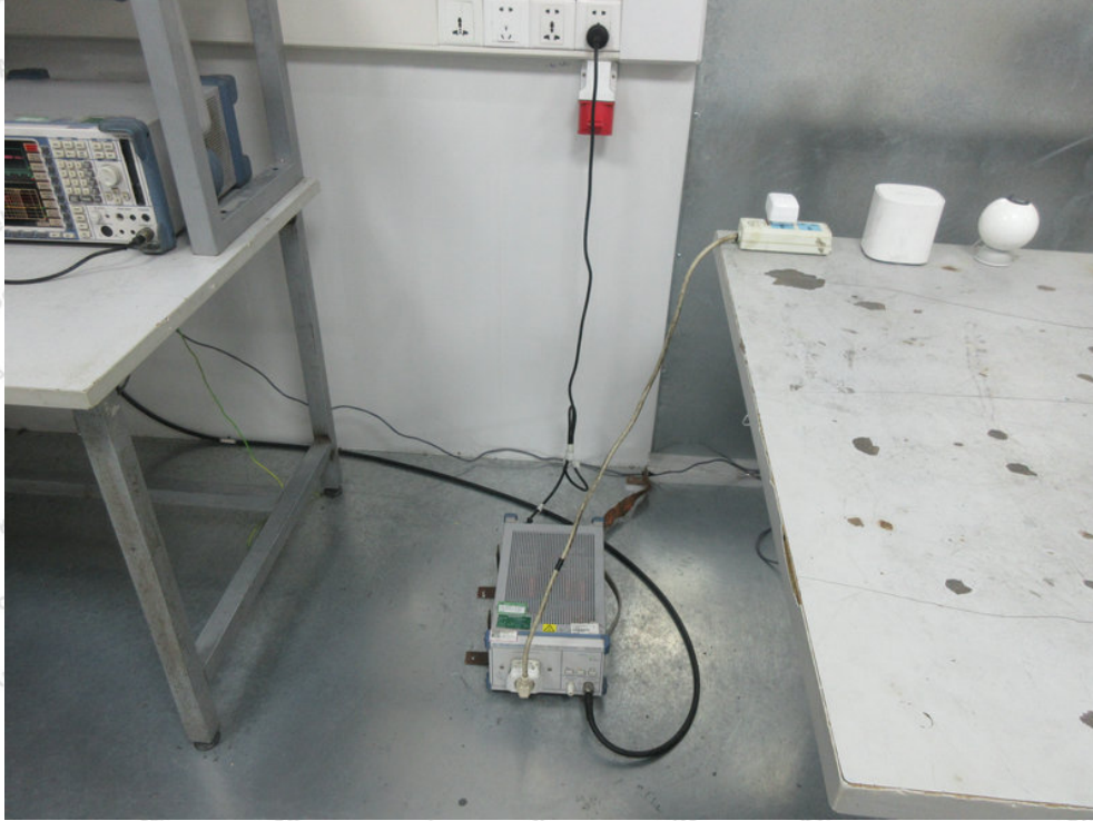
Photo of Conducted Emission Measurement
