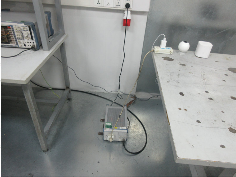
Photo of Power Line Conducted Emission Test
