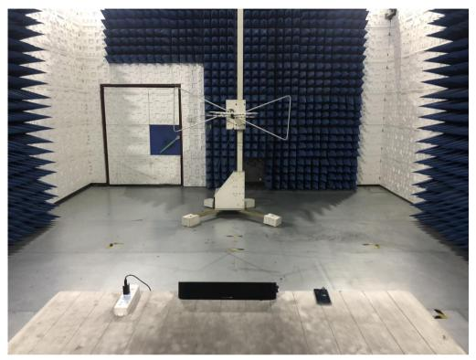
RADIATED EMISSION TEST SETUP ABOVE 1GHZ
