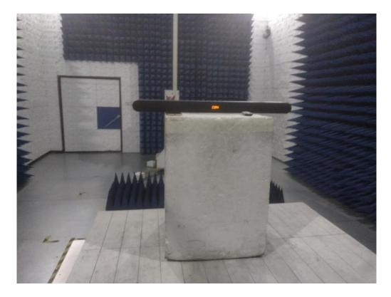
CONDUCTED EMISSION TEST SETUP-FRONT
