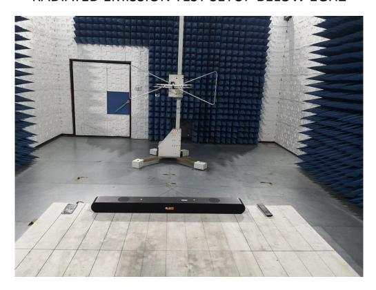
RADIATED EMISSION TEST SETUP BELOW 1GHZ-BACK
