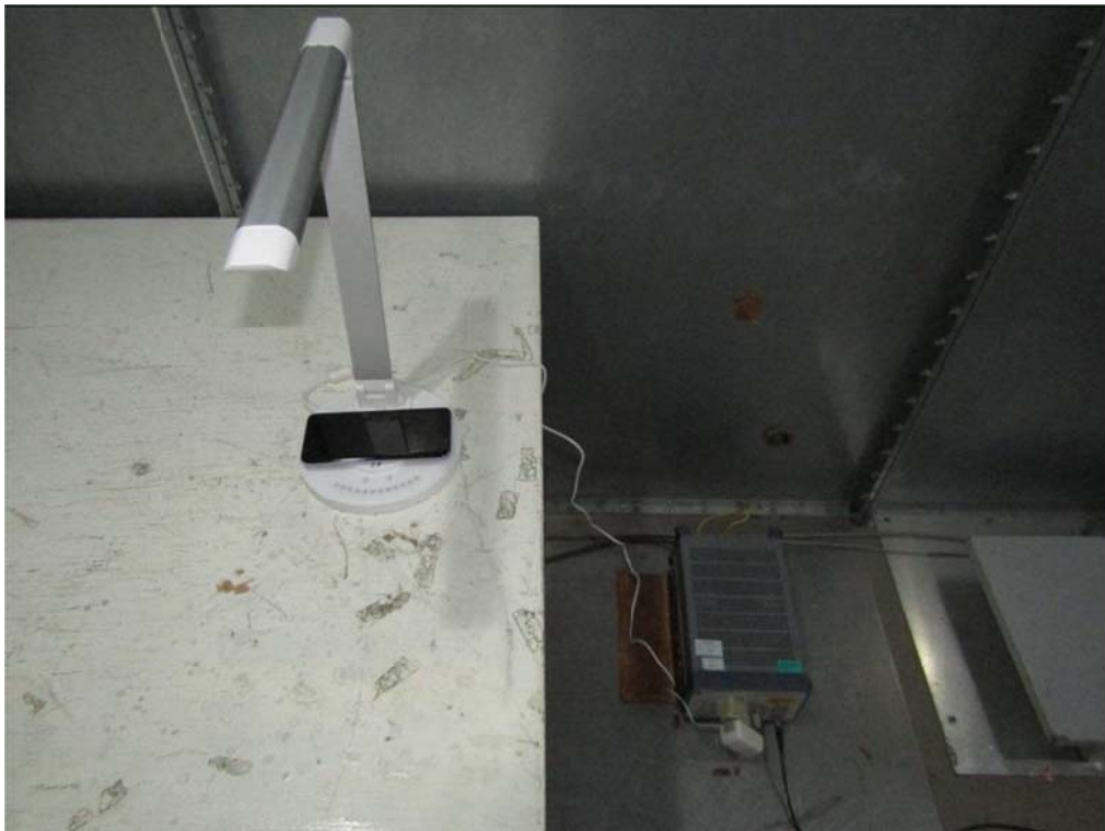
Measurement of Conducted Emission Test Set Up
