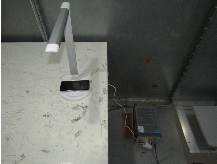
Measurement of Conducted Emission Test Set Up
