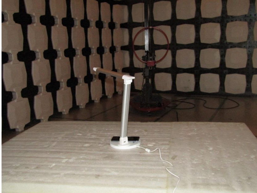
Measurement of Radiated Emission Test Set Up
