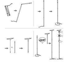
Note: • Remove the plastic rings before installing the lamp. • When connecting the lamp sections with the base or the lamp head, • When connecting the lamp sections with the Source with too much force. If it gets stuck, undo and restart again. • Align the male connector with the female connector, then click and ratate 90° or 270° to lock in place.
