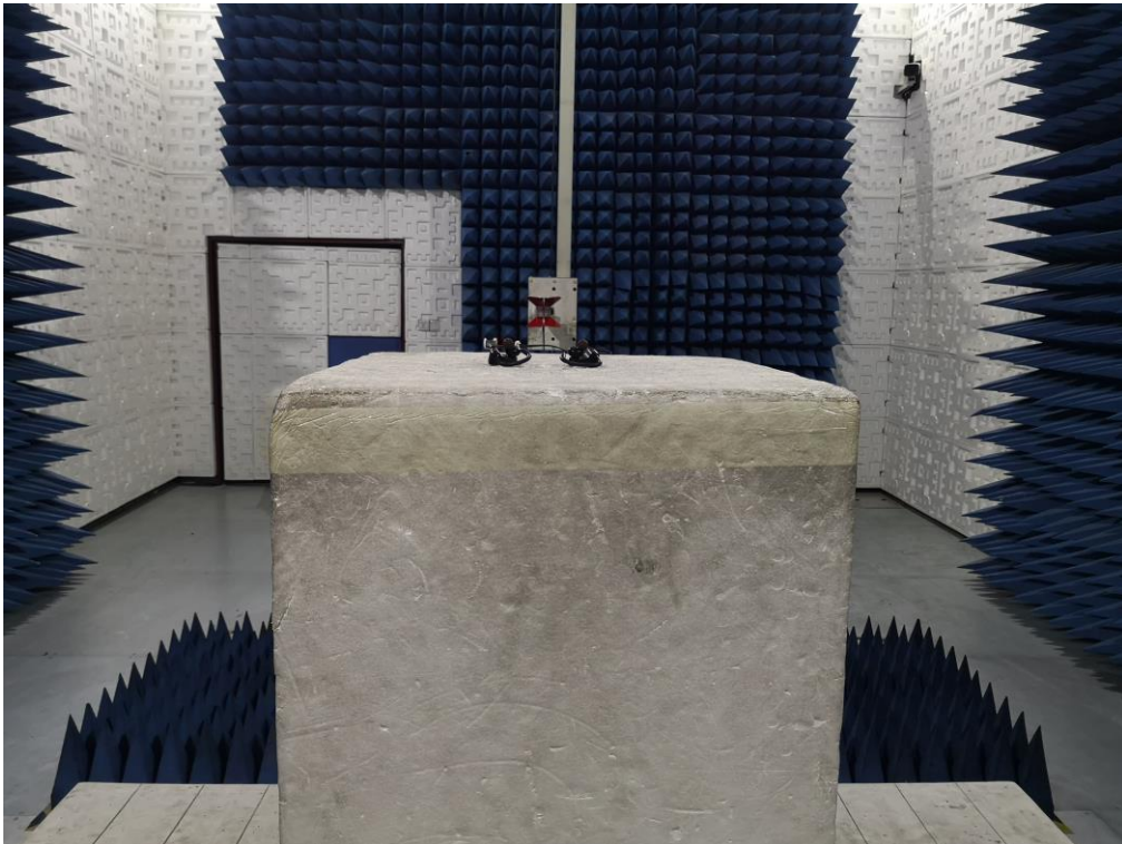
RADIATED EMISSION TEST SETUP ABOVE 1GHZ
