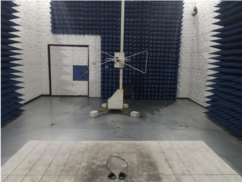
RADIATED EMISSION TEST SETUP ABOVE 1GHZ
