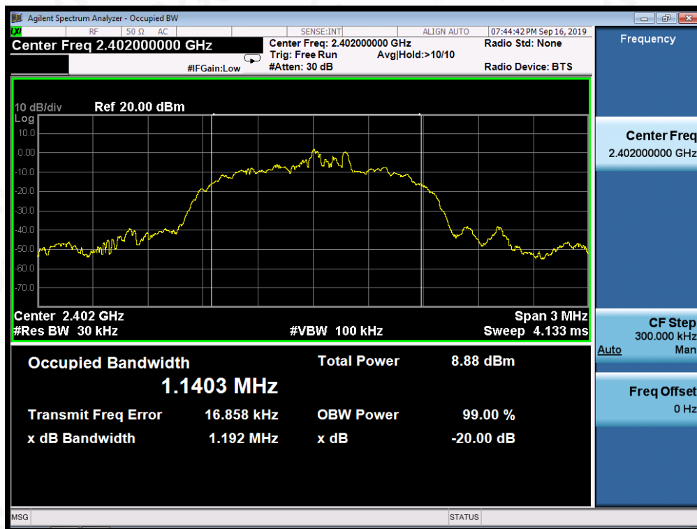
TEST PLOT OF BANDWIDTH FOR LOW CHANNEL
