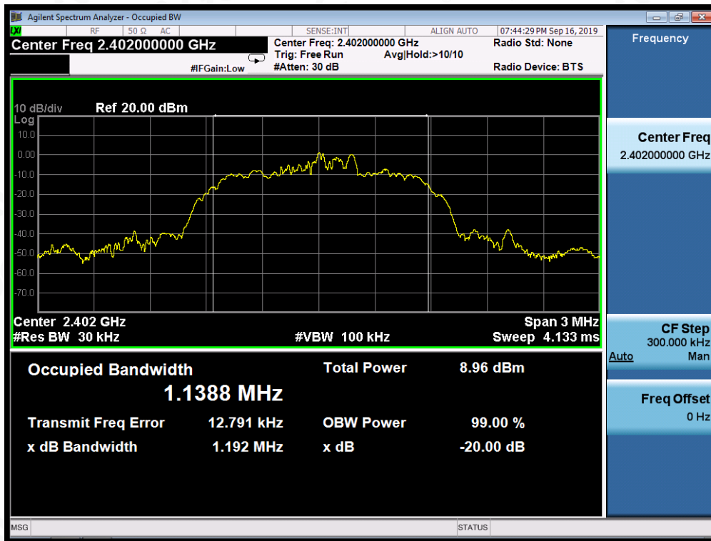
TEST PLOT OF BANDWIDTH FOR LOW CHANNEL
