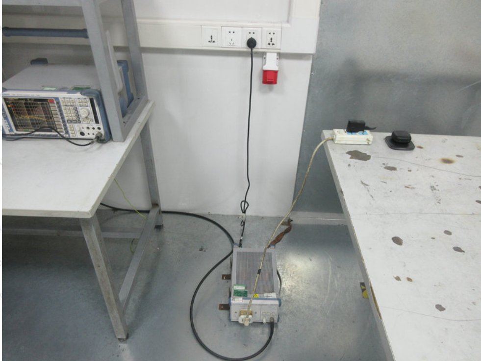
Photo of Conducted Emission Measurement
