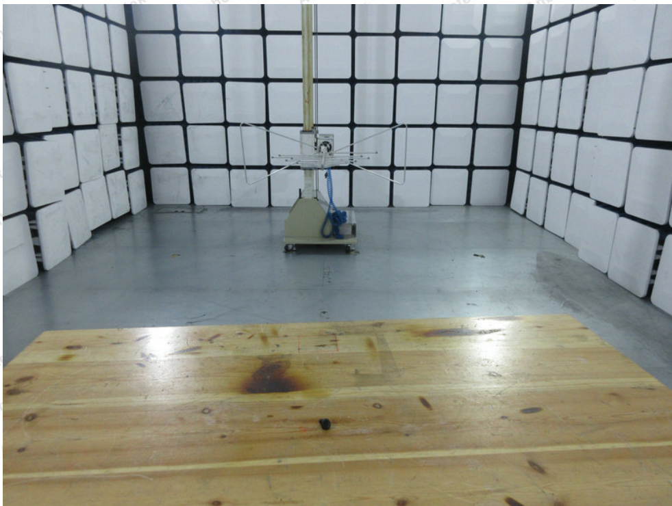
Photo of Radiation Emission Test
