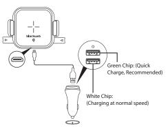
1. Connect the micro USB cable into the charging port.
