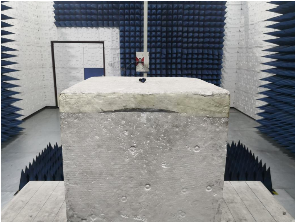
RADIATED EMISSION TEST SETUP ABOVE 1GHZ
