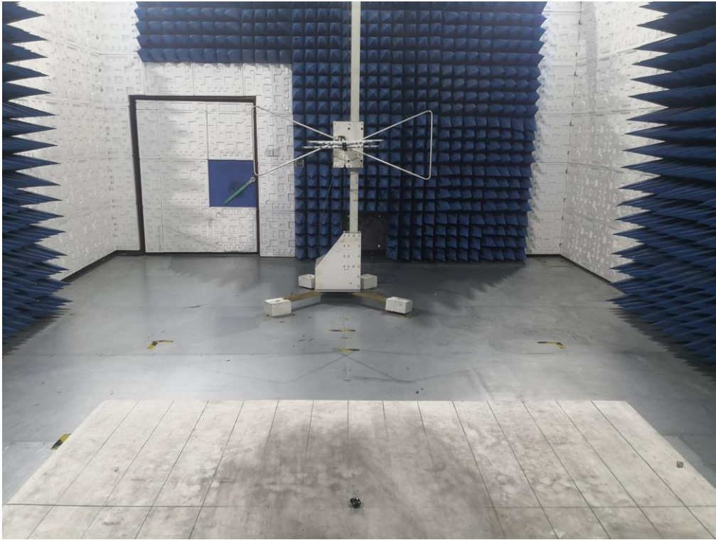
RADIATED EMISSION TEST SETUP ABOVE 1GHZ
