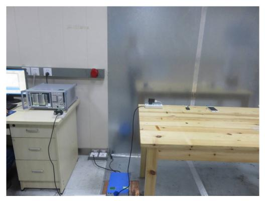
FCC RADIATED EMISSION TEST SETUP
