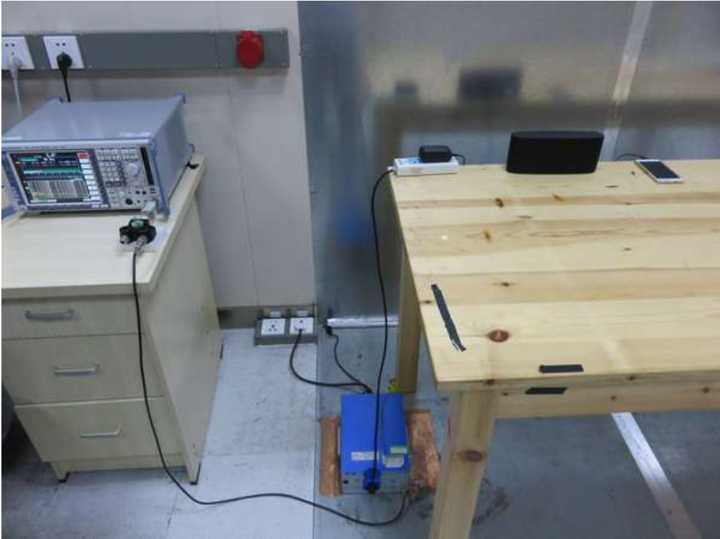
FCC RADIATED EMISSION TEST SETUP
