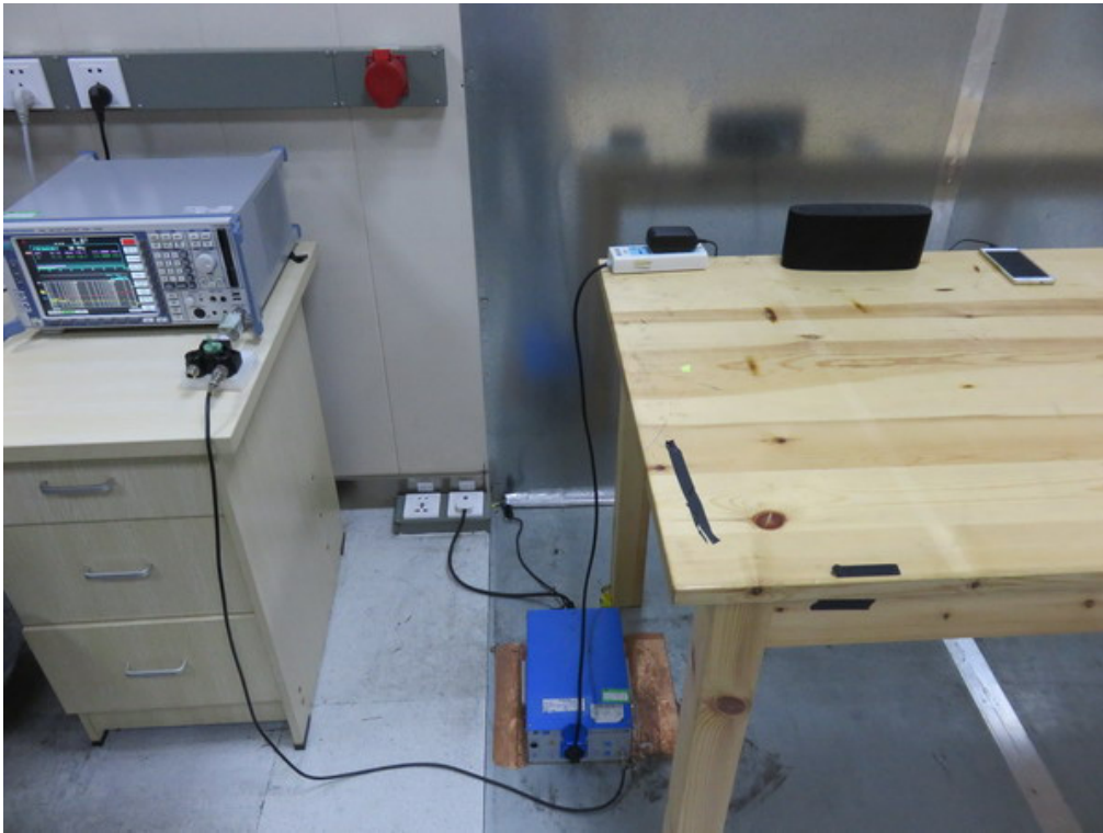
FCC RADIATED EMISSION TEST SETUP
