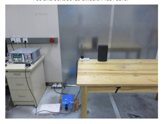
FCC RADIATED EMISSION TEST SETUP
