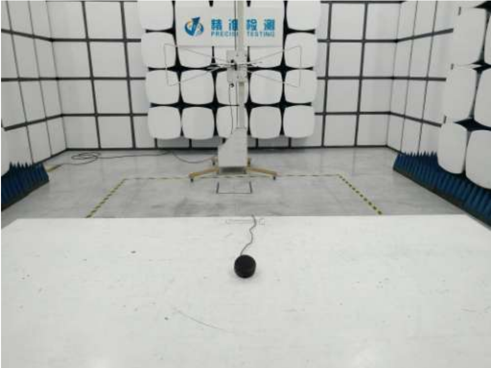
FCC RADIATED EMISSION TEST SETUP ABOVE 1GHZ
