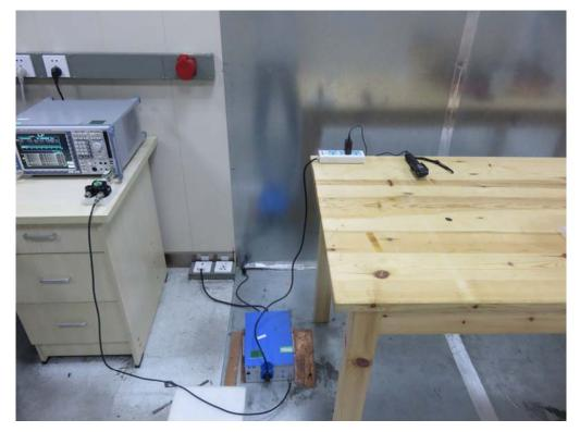
FCC RADIATED EMISSION TEST SETUP
