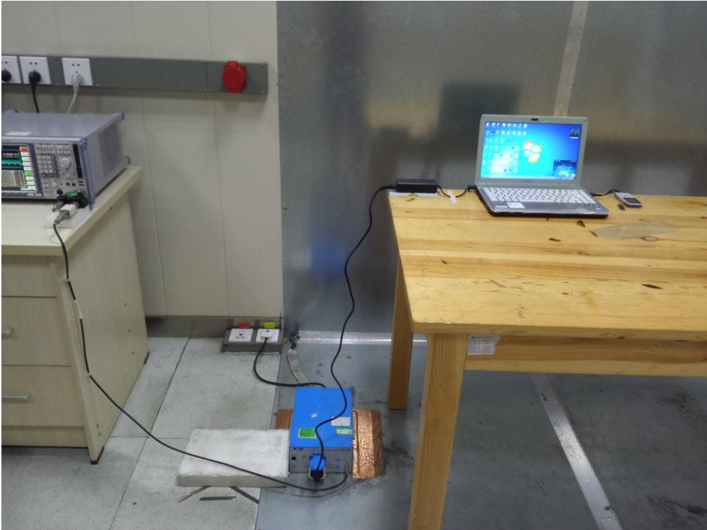
FCC RADIATED EMISSION TEST SETUP
