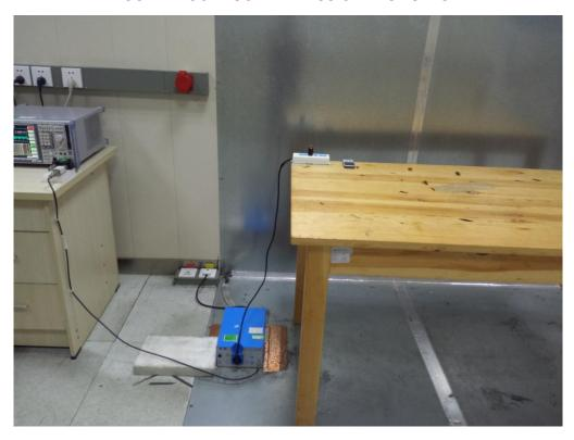
FCC RADIATED EMISSION TEST SETUP
