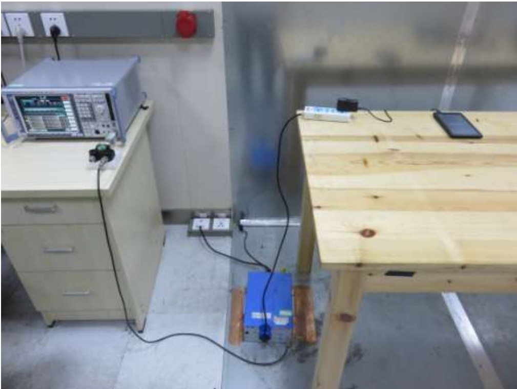
FCC RADIATED EMISSION TEST SETUP
