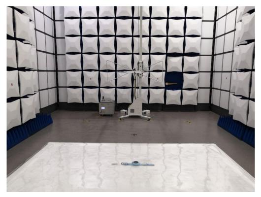
RADIATED EMISSION ABOVE 1G TEST SETUP
