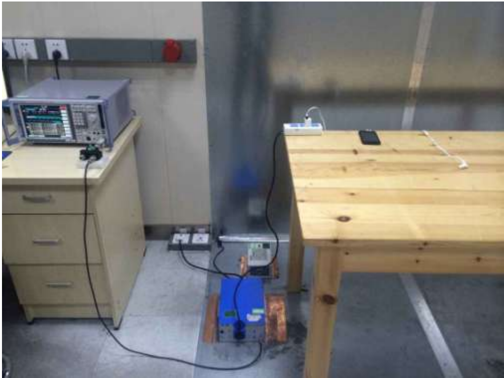
FCC RADIATED EMISSION TEST SETUP
