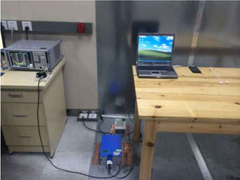
FCC RADIATED EMISSION TEST SETUP
