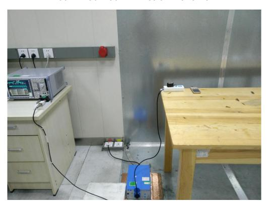
FCC RADIATED EMISSION TEST SETUP
