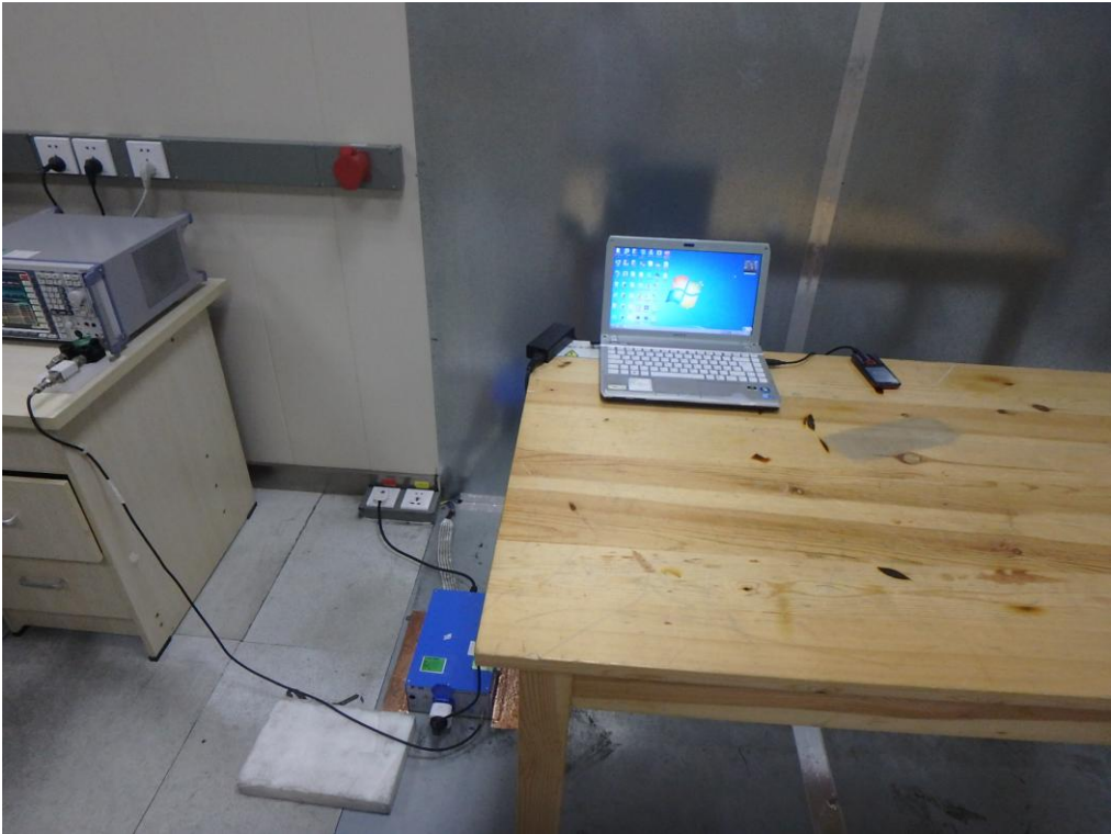
FCC RADIATED EMISSION TEST SETUP
