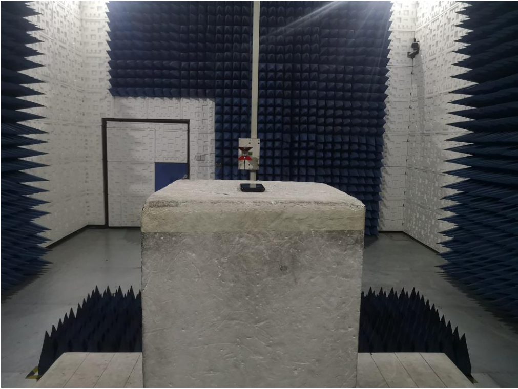
RADIATED EMISSION TEST SETUP ABOVE 1GHZ
