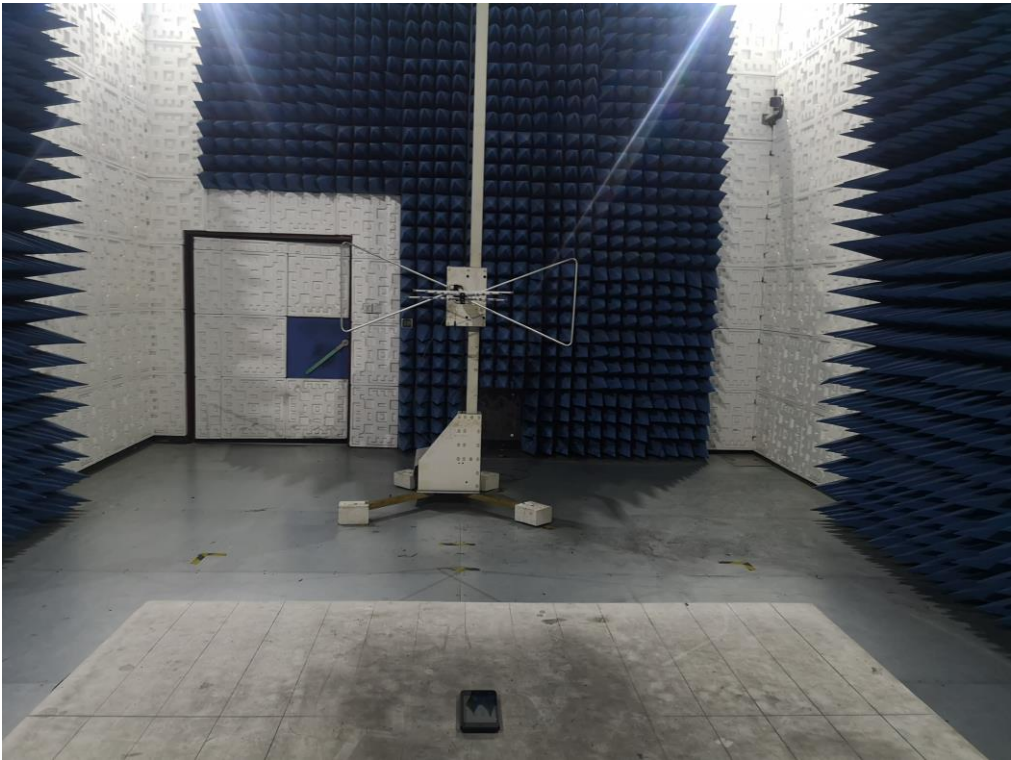
RADIATED EMISSION TEST SETUP ABOVE 1GHZ
