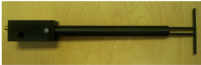
Figure 1 – MVG COMOSAR Validation Dipole
