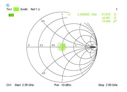
Calibrated return loss: -29.54dB; Measurement return loss: -29.55 dB(within 20%)
