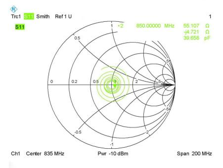
Calibrated return loss: -24.51dB; Measurement return loss: -24.34 dB(within 20%)
