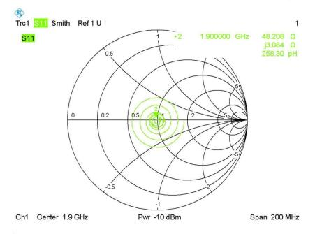
Calibrated return loss: -27.75dB; Measurement return loss: -28.32 dB(within 20%)
