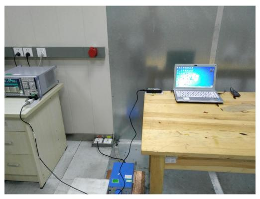
FCC RADIATED EMISSION TEST SETUP
