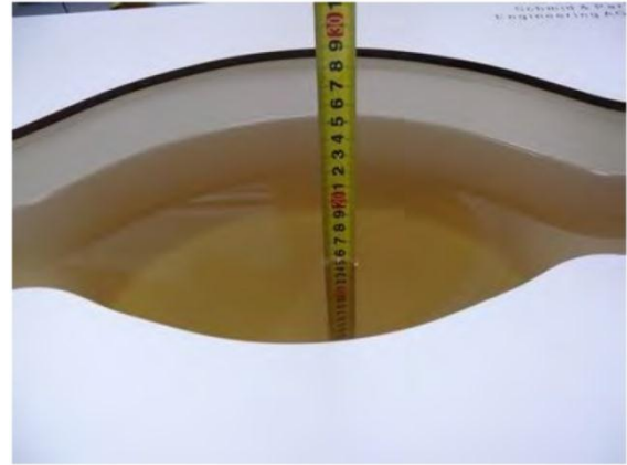
Liquid depth in the body phantom (835MHz)
