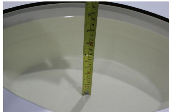
Liquid depth in the body phantom (1900MHz)
