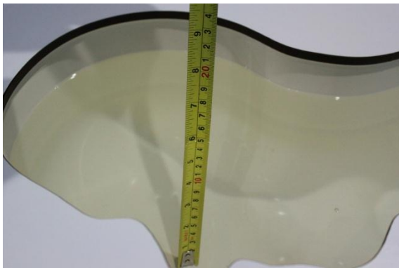
Liquid depth in the head phantom (1900MHz)
