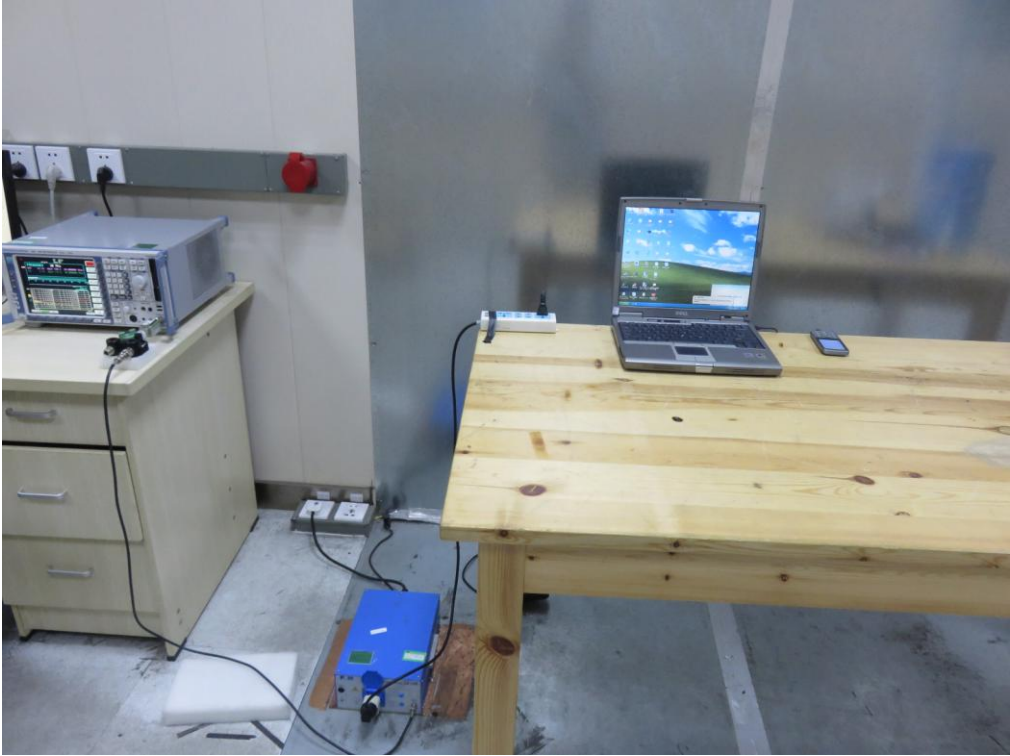
FCC RADIATED EMISSION TEST SETUP
