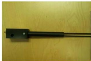
Figure 1 – MVG COMOSAR Validation Dipole
