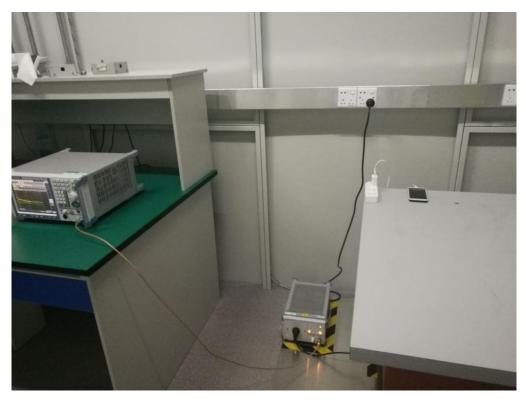
RADIATED EMISSION TEST SETUP
