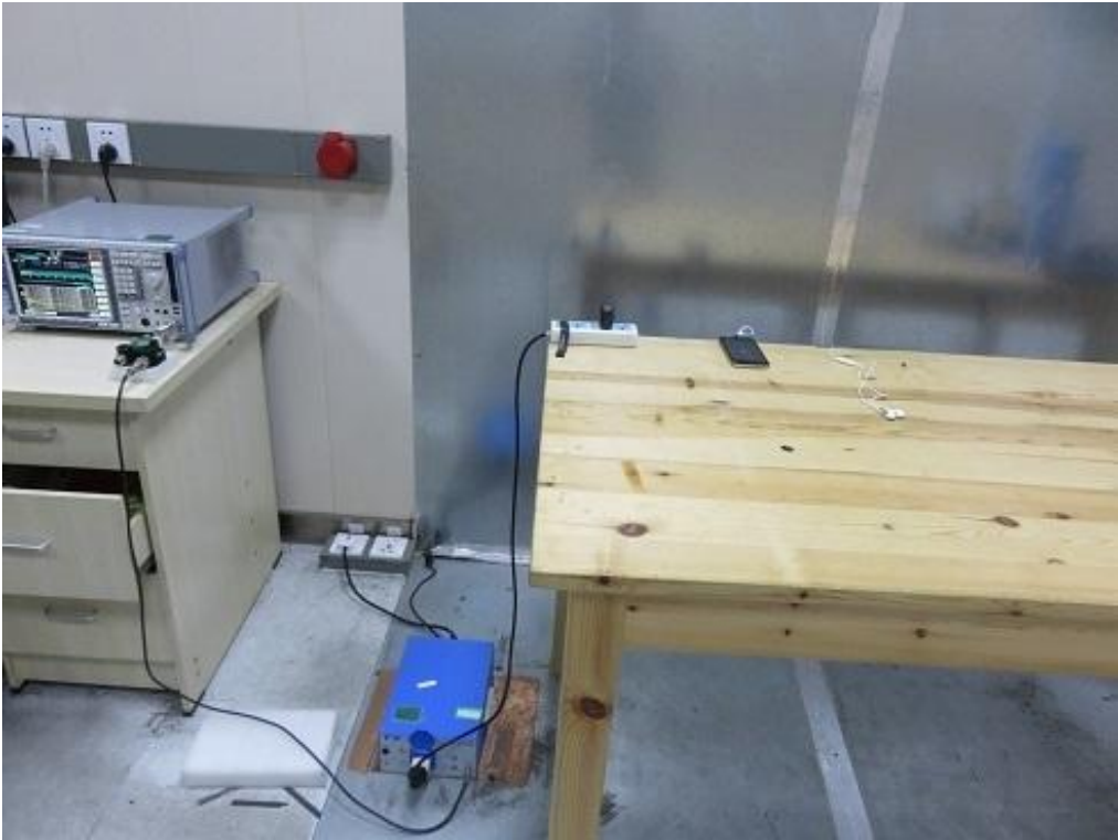
FCC RADIATED EMISSION TEST SETUP
