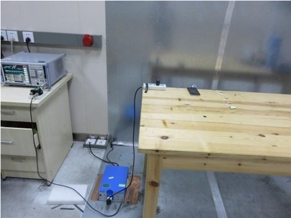
FCC RADIATED EMISSION TEST SETUP
