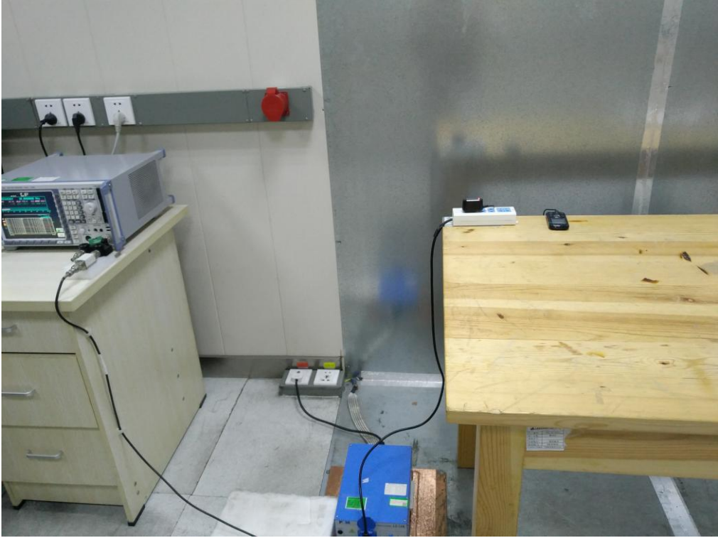
FCC RADIATED EMISSION TEST SETUP
