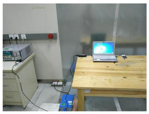
FCC RADIATED EMISSION TEST SETUP
