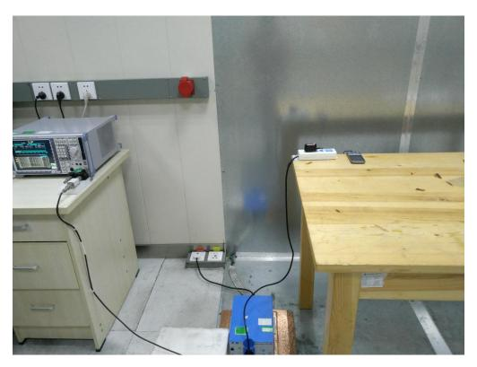
FCC RADIATED EMISSION TEST SETUP
