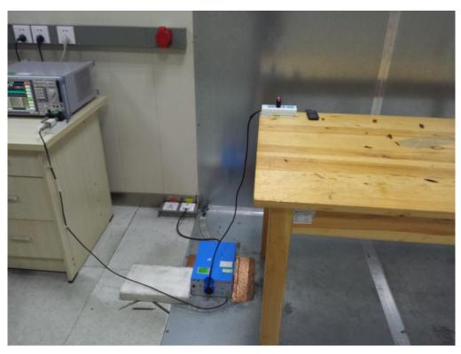
FCC RADIATED EMISSION TEST SETUP
