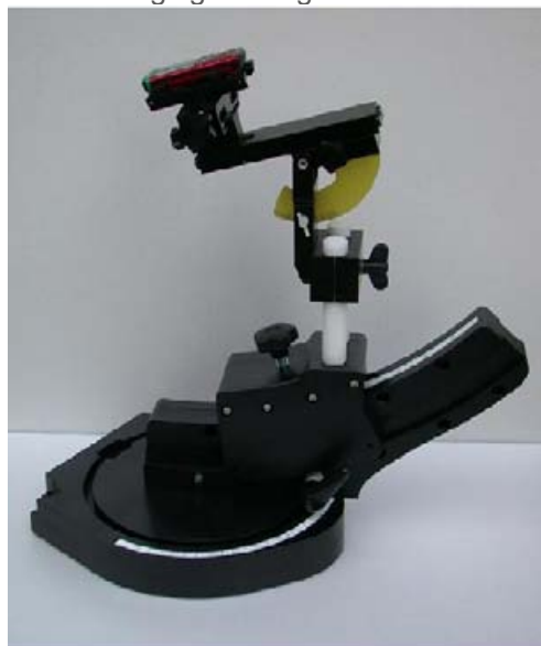
Device holder supplied by SPEAG
