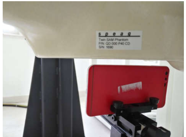
Hotspot mode - Right Side (10mm)
