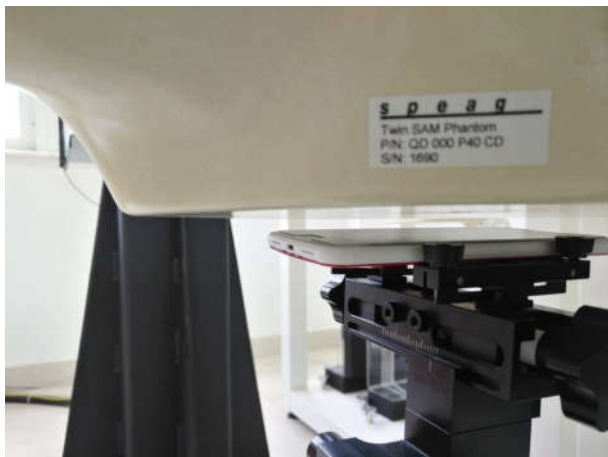
Body-worn Front Side (10mm)
