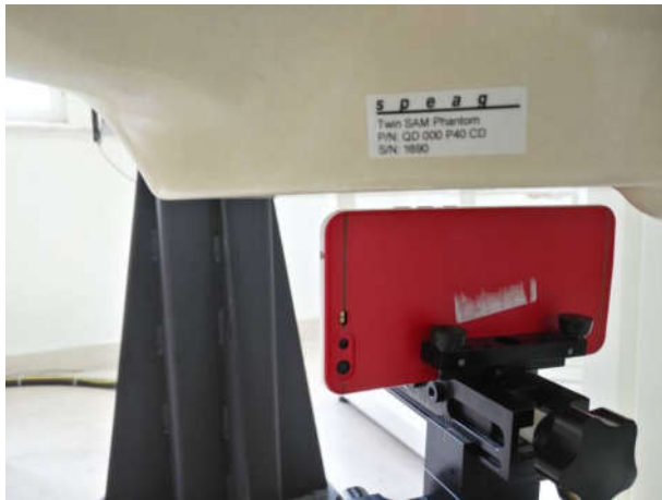
Hotspot mode - Left Side (10mm)
