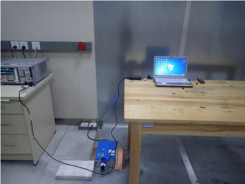
FCC RADIATED EMISSION TEST SETUP
