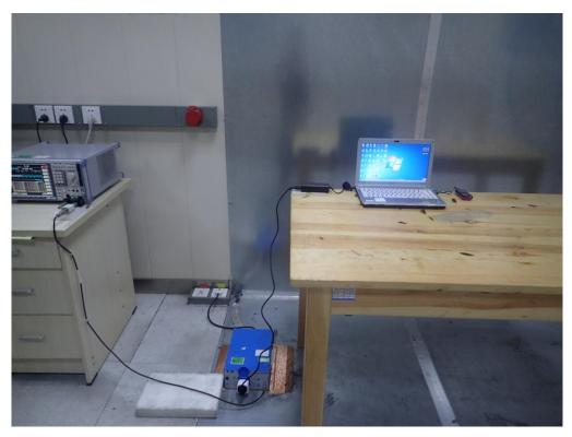
FCC RADIATED EMISSION TEST SETUP
