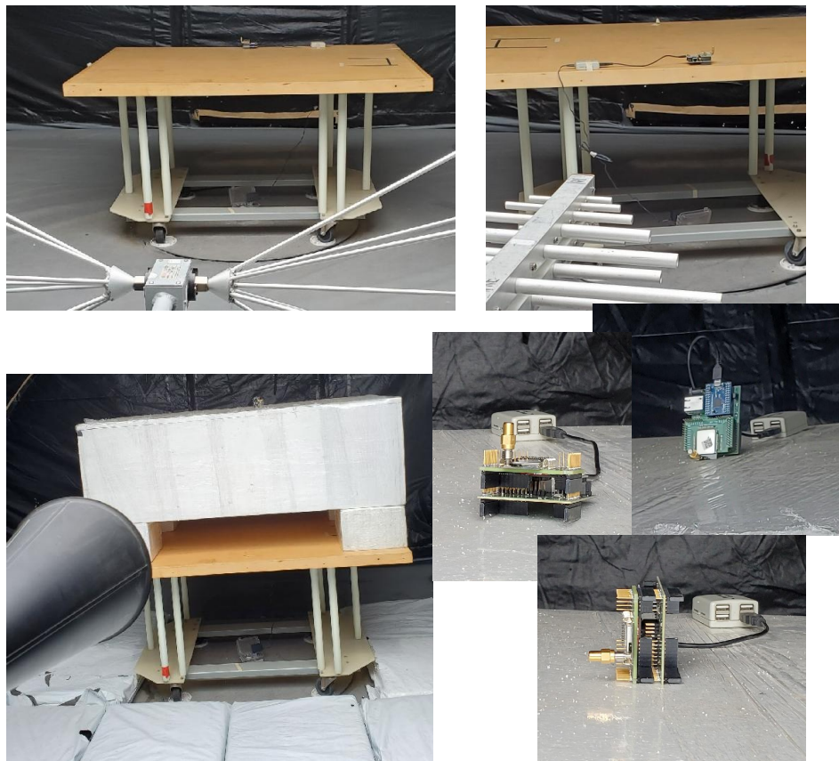
Figure 4: Radiated Emissions Test Setup Photograph(s).
