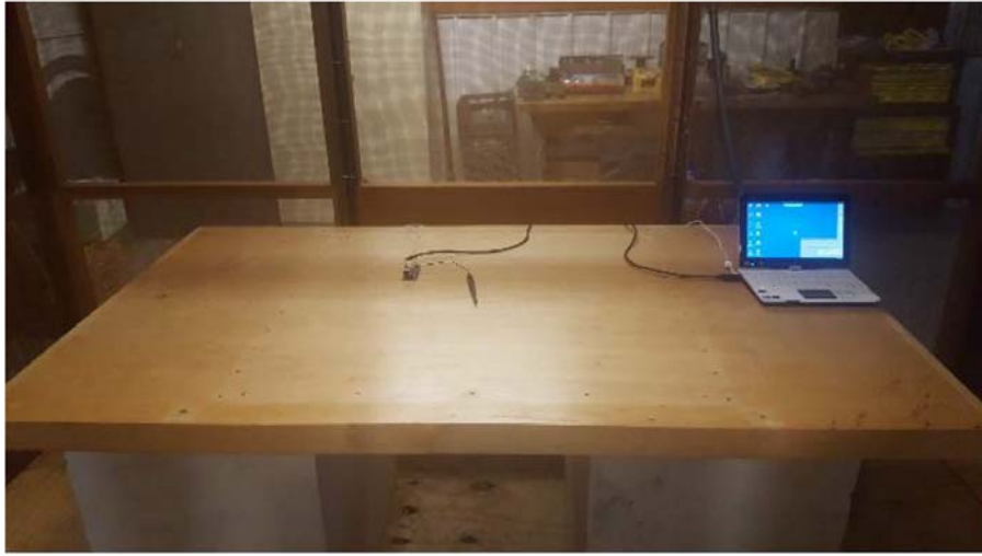
Figure 7: Conducted Emissions Test Setup Photograph(s).
