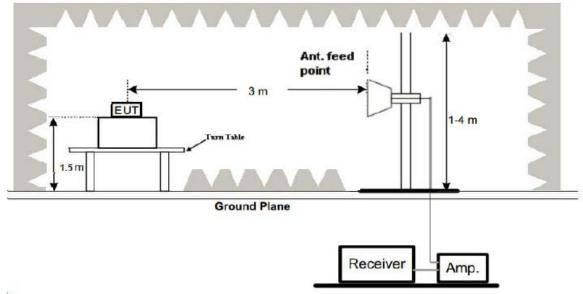
(3) Radiated Emission Test-Up Frequency Above 1GHz
