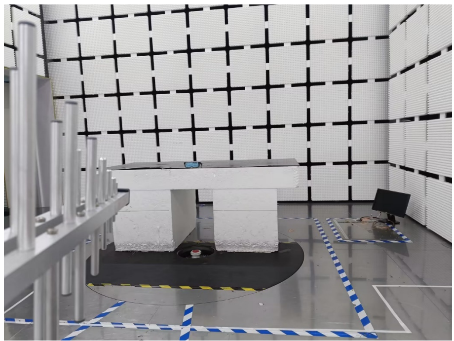
Radiation Emission Test Setup (30MHz to 1GHz)
