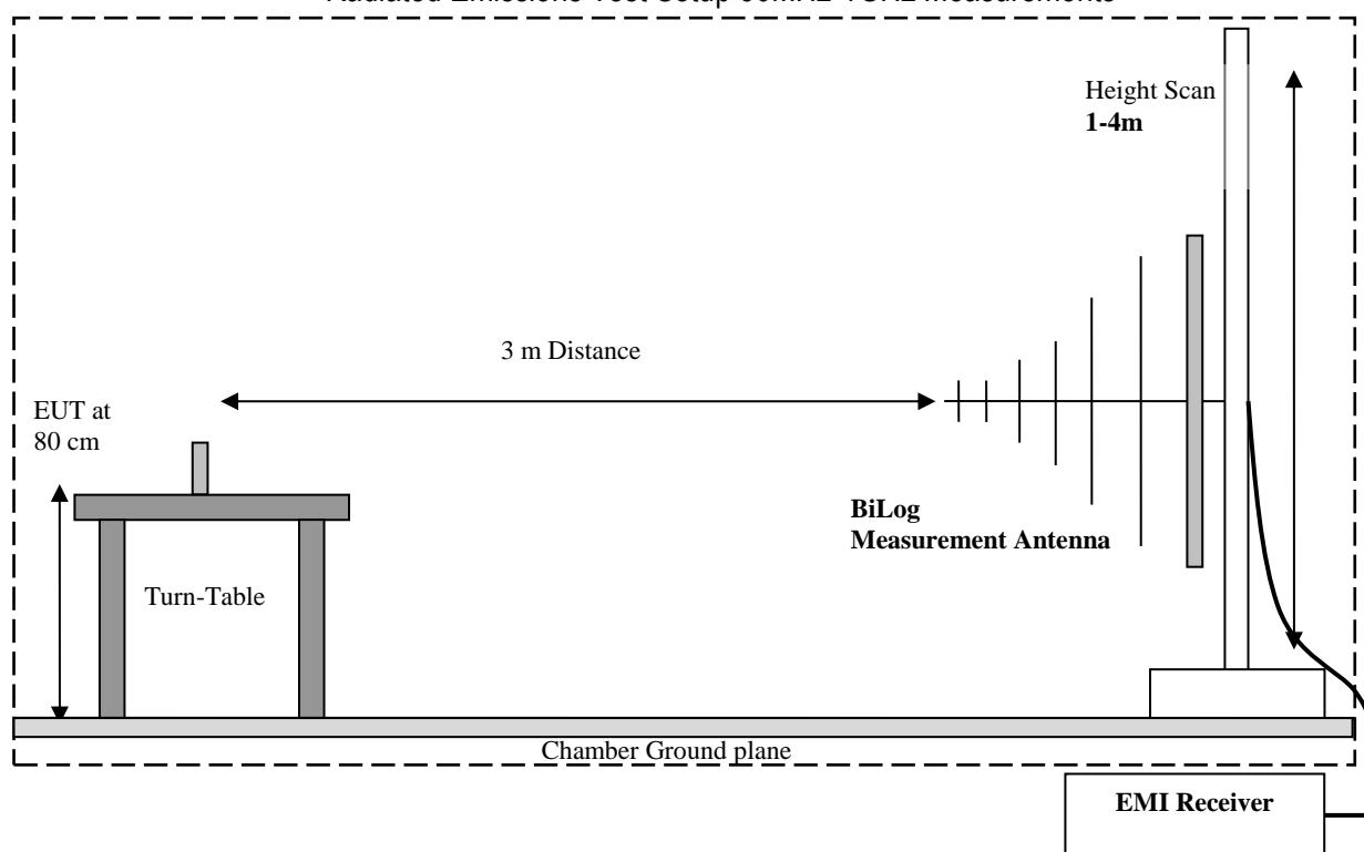
**Radiated Emissions Test Setup above 1GHz Measurements**
